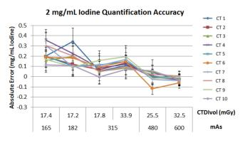
2mg/mL iodine rod quantification accuracy by mAs for 10 fast-kVp switching Multi-Energy CT scanners. Accuracy averaged over a 1 year period.
