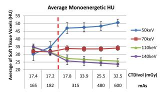
Average soft tissue monoenergetic HU for 50, 70, 110, and 140 keV reconstructions versus mAs, averaged over a 1 year period. Protocols left of the red dashed line were insufficient to provide reliable HU values.
