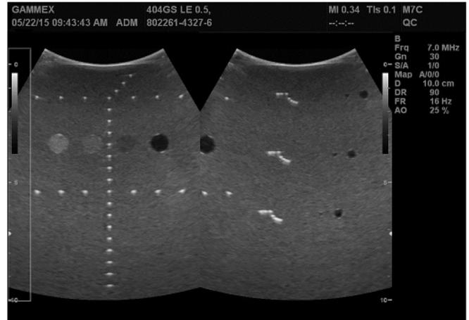
Closely spaced pin targets are ideal for testing high frequency transducers.
