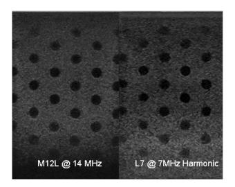
The Sono408 Phantom incorporates both 2mm and 4mm diameter tissue mimicking spherical lesions which lie in a single plane at the center of the phantom.
